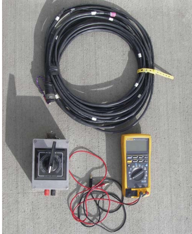
Figure 2: Thermistor Cable Array Setup
