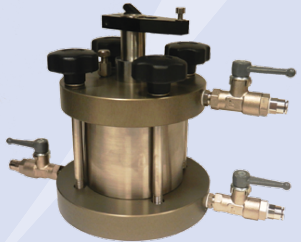
VJT0680 - Constant Rate of Strain Cell (75.7 mm) diameter
