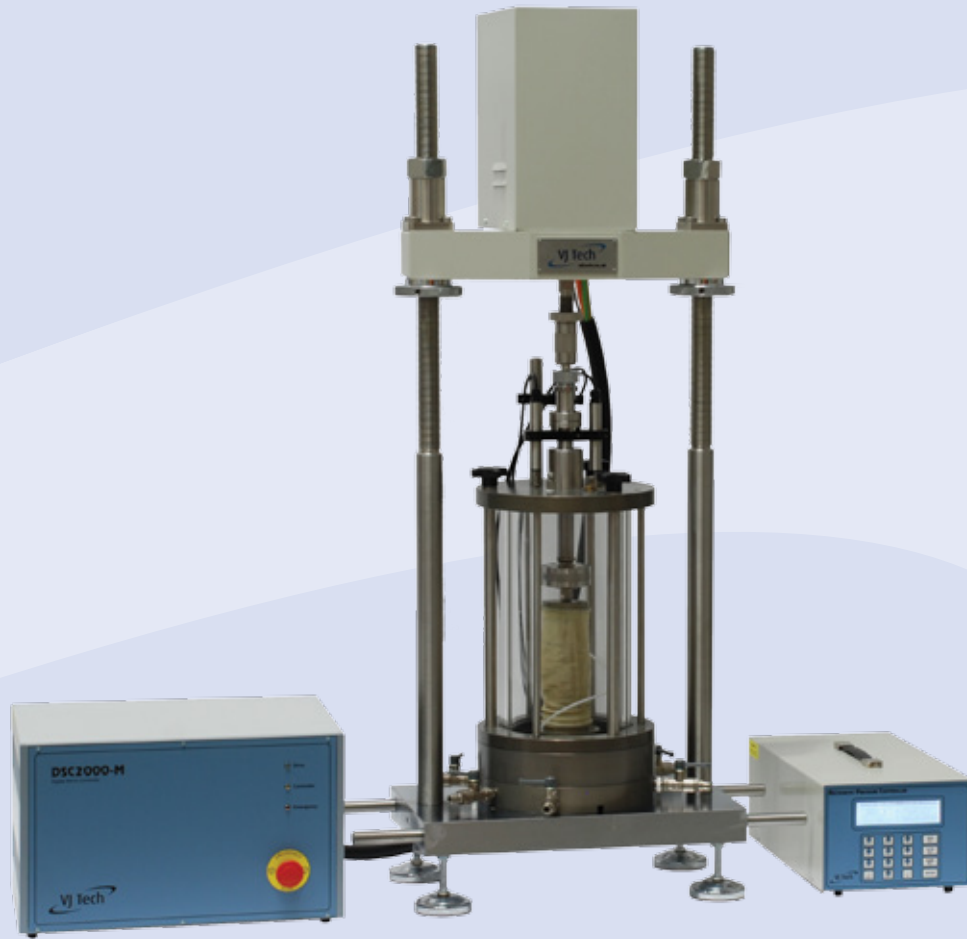
VJT9406 - Dynamic Resilient Modulus Testing System
