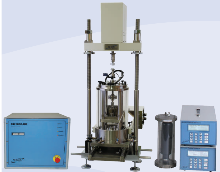
VJT9411 - Dynamic Simple Shear with Confining Pressure Testing System
