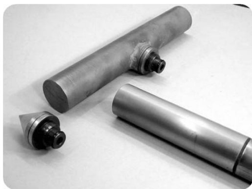
Figure 4. Picture of cone penetrometer and T-bar used at Onsøy.
