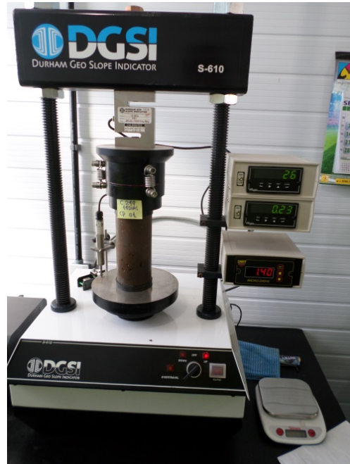
Fig. 6 Unconfined compression test
