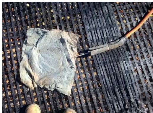
Fig.11 photo. Load cell installed on top soil between columns
