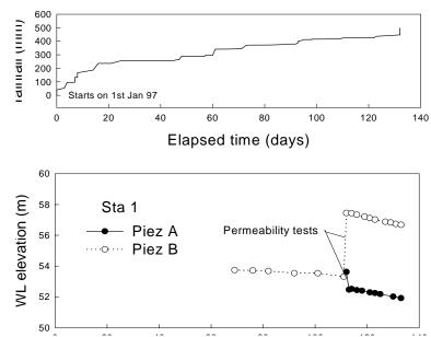
Figure 7 (a) Rainfall, water level and (b) permeability tests
