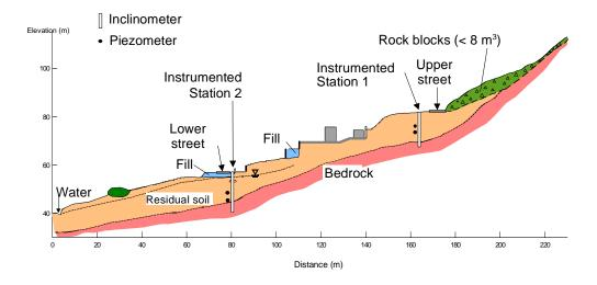
Figure 2 Cross section BB'
