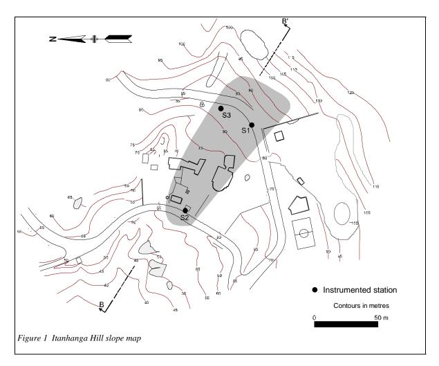
the following investigations were conducted: geophysical and topographic surveys, geological photo interpretation and field surface mapping, boreholes and automated field instrumentation.
