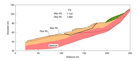
Figure 3 Results from the stability analyses
