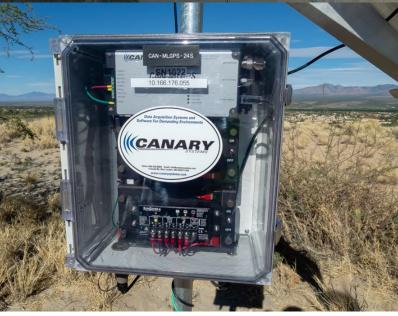
The Canary Systems® MLGPS® integrates a multifunction GPS module into a turnkey power control, battery charging and communications platform, specifically designed for geotechnical and structural monitoring applications. It is available in several costeffective variants including a portable version for quick deployments, and a fixed version for permanent deployments. All MLGPS units feature a NEMA rated enclosure, battery, and solar panel.
