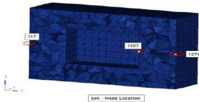
Figure 7. Soil node location around concrete chamber.
