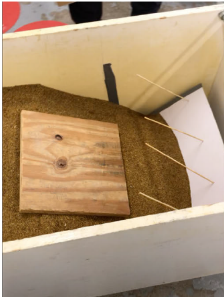
Figure 4 – ENU Experiment – Pull-out Failure
