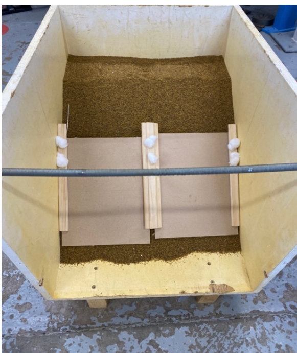
Figure 13.0 Failure of the retaining wall built
