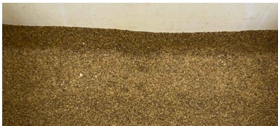
Figure 2.0- Leighton Buzzard silica sand
