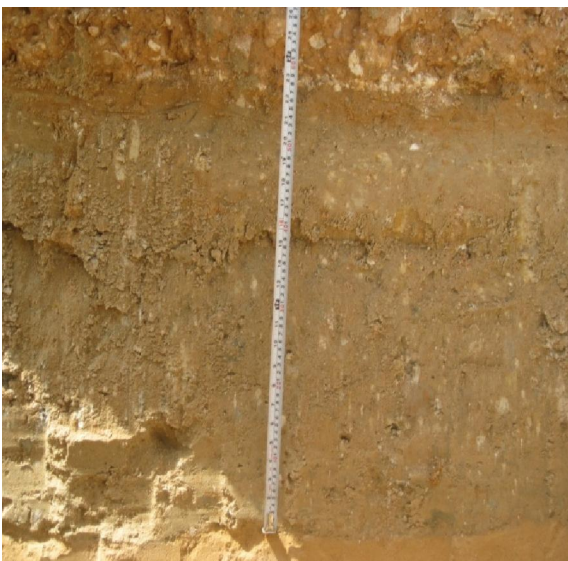
Figure (4): Collapsible Soils Under the Base Layer
