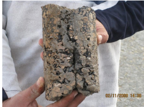
Figure (3): Core Sample on Cracks Shows Deep Cracks Along Sample
