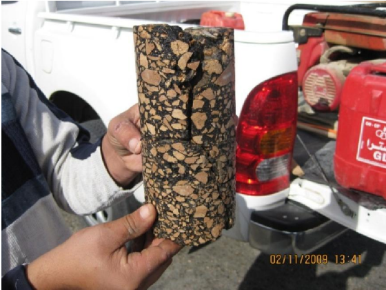
Figure (3): Core Sample on Cracks Shows Deep Cracks Along Sample
