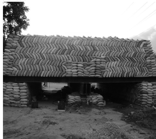
Fig. 1 Shows the pile load test
