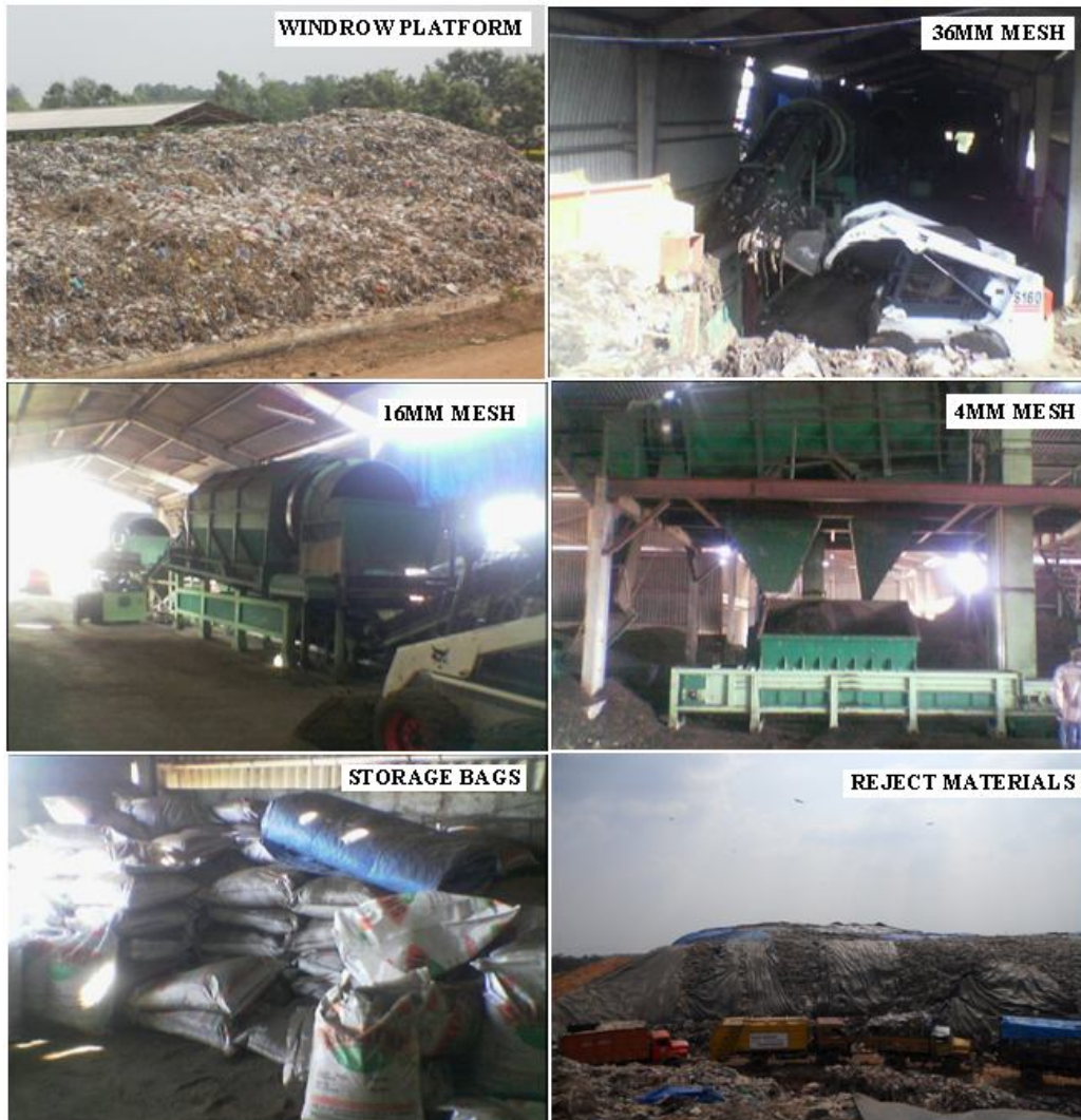
Fig 3. Windrow composting process
