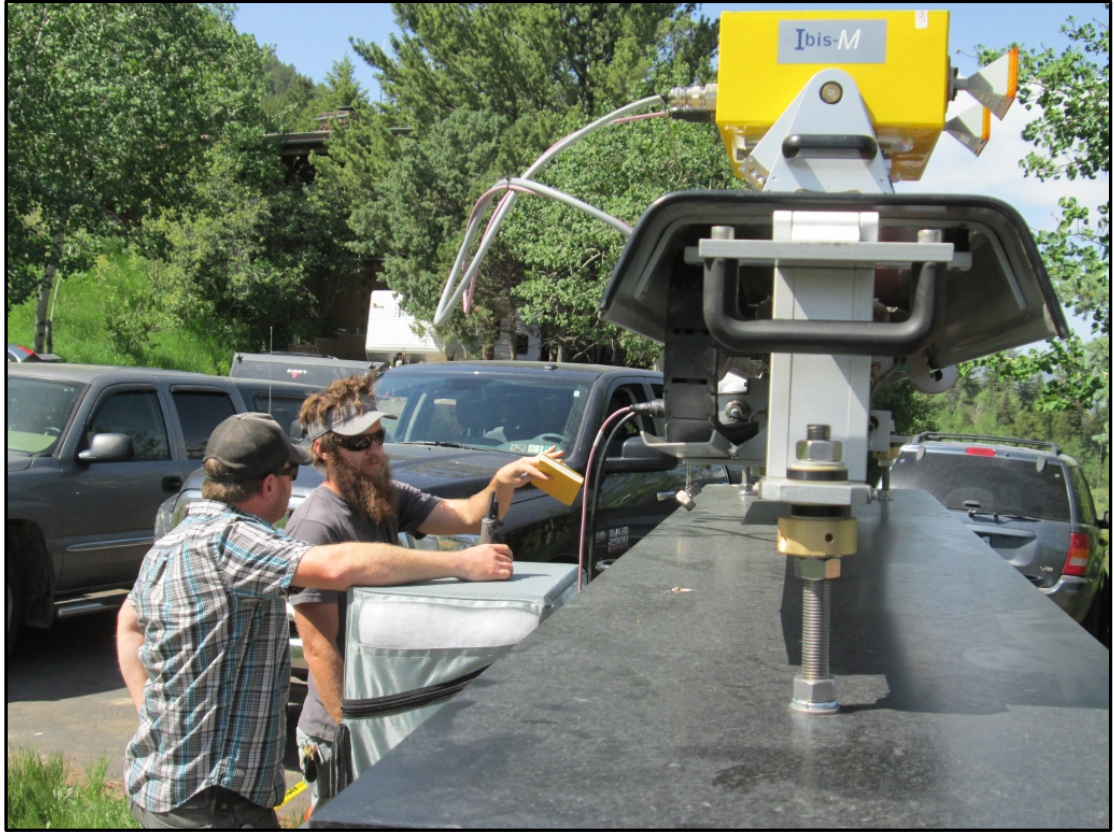
Fig. 2: Cliff and Jason read-in the coordinates at the radar position. Data is geocoded and can be associated with other datasets. Guardian software allows the inclusion of point data from other instruments. The current project scan area includes the slide area from the rooftop of Walgreens, to the peak of Gros Ventre Butte.
