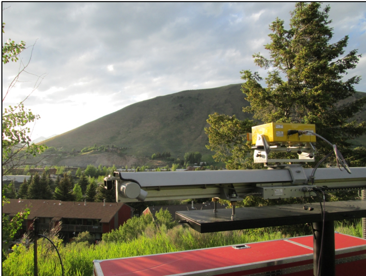
Fig. 1: IBIS-FM unit scanning across the valley towards the Gros Ventre Butte. Data returns have good coherence and information is being collated every 5 minutes (1 scan). Following the completion of two scans, displacements are recorded and plotted against time. Scanning began about 19:00 Thursday evening.
