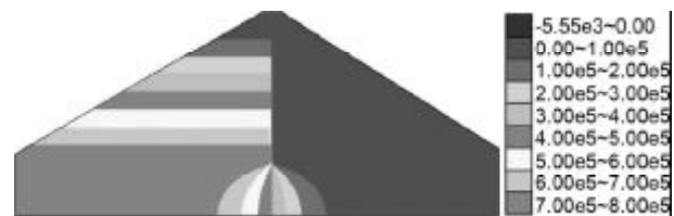
Figure 5. Pore pressure contours after impounding.
