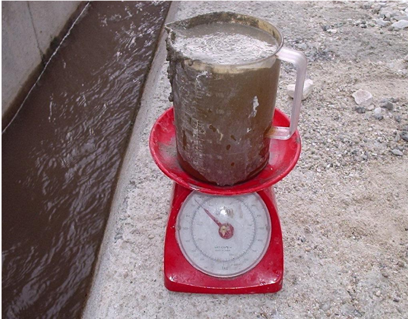
Density monitoring of foamed concrete
