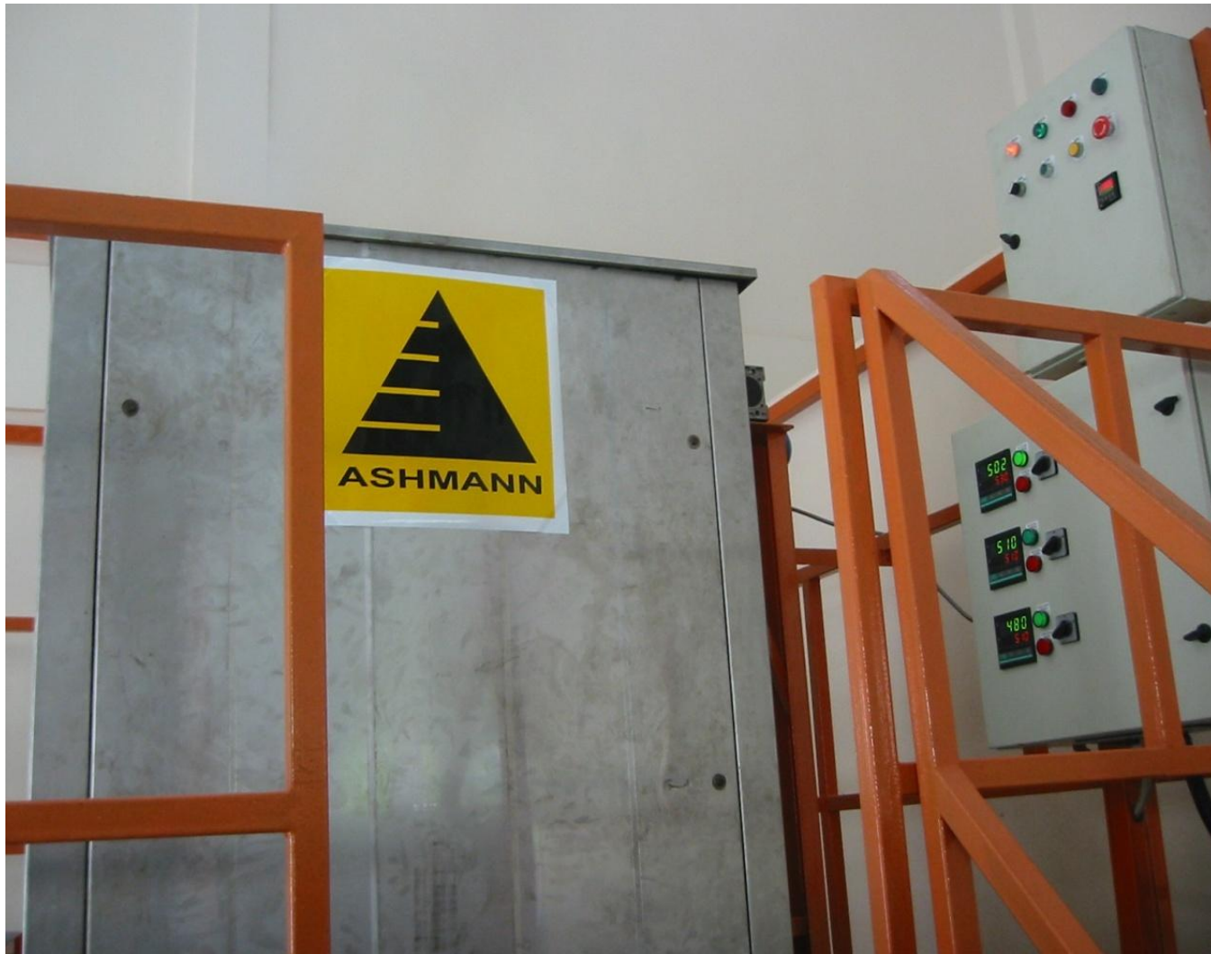
Reactor furnace for amorphous biomass silica ash synthesis
