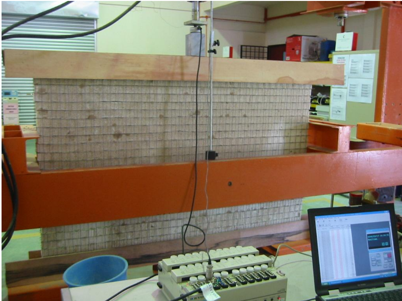
KUiKwall component tested for load bearing capacity
