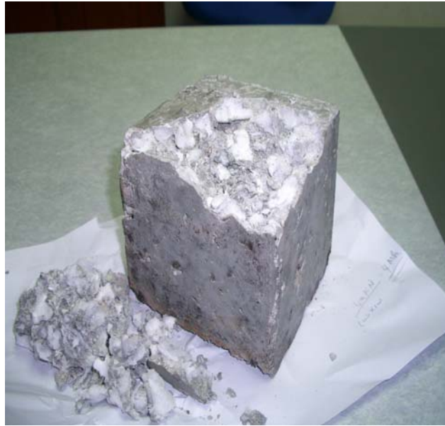
Figure 5: Compression test samples of lightweight Styrofoam aggregate concrete
